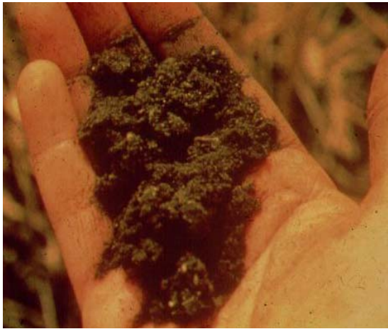
Figure 3. Sludge removed from Reed Bed following many years of operation.
